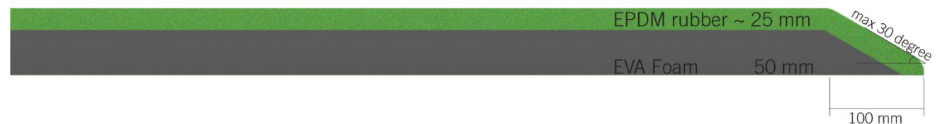
Type 3 Detail view of the Floor with 50 mm shock absorbing
